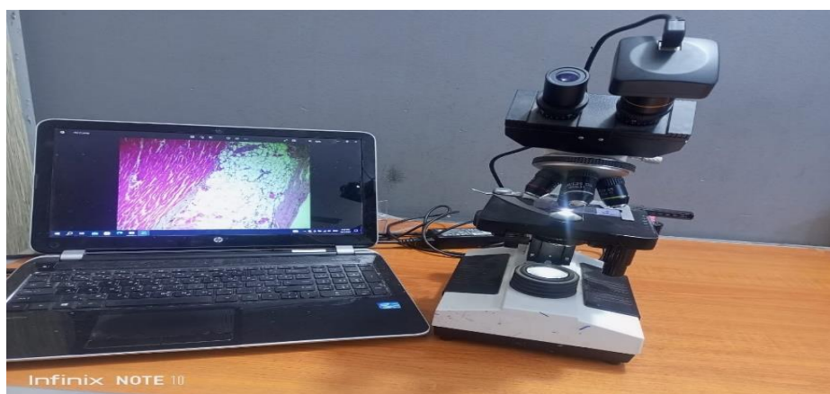
Figure(2): shows light microscope type (XSZ-107bn) and camera AM scope mu 300.
