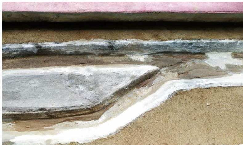
2nd Figure. Merging of two channels at an angle of \alpha = 45^\circ
