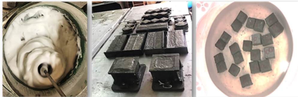
Figure 1. Casting details to cast and curing ,test the compressive strength and flexural strength for different volume carbon fiber and Pour the optimal mixture by 1% Nano slice and carbon fibers and curing in water at 7 and 28 days
