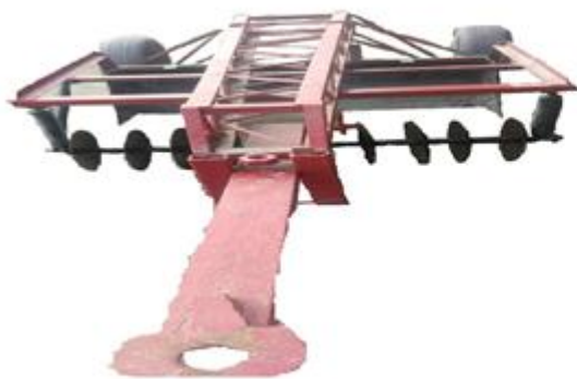
Figure 3. The process of working the ground rectifier with a base on which the device with a softening disc is installed.
